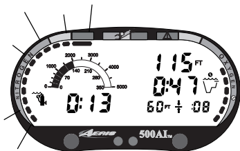
Fig. 71 - Delayed Violation (> 60 FT ceiling required)
